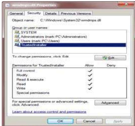
Figure 16: The Trusted Installer has full control
